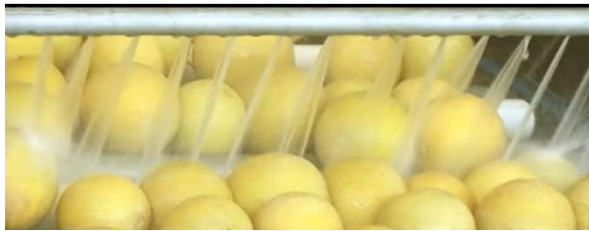
Detail of the melon wash process, and image of the packing house. Water used in the process is recirculated, and contains Peroxide UltraPure™ that keeps it clean.
