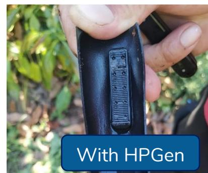
*Comparison of drippers in sectors without HPGen, and with HPGen. The brown substance in the picture without HPGen was determined to be bacterial slime. This blocks the water path in the dripper, and causes poor irrigation uniformity. The dripper with HPGen dosing appears very clean, without any obstructions on the water path.*
